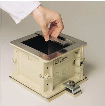
Verification of a cube mould with Go/No go gauges
