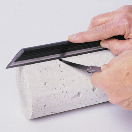
Straightness verification of cylinder generatrix using straightedge and feeler strips
