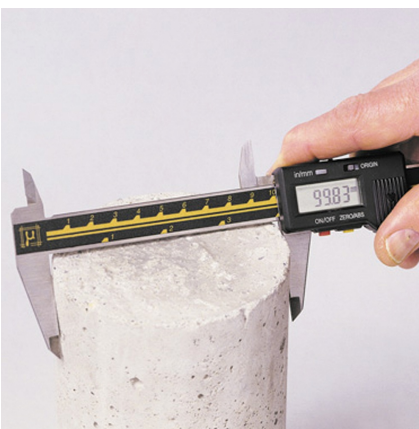
Verification of diameter using digital vernier caliper
